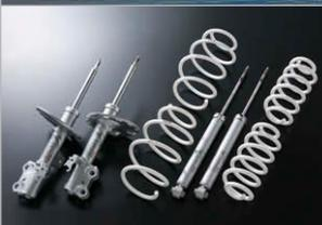
KYB has introduced a feature that makes the damping-force adjustable over 32 levels (for some models, eight levels of adjustment with the rear shock absorber). This new feature makes it possible to choose an optimal setting for the damping-force, which varies according to the tires used and the kind of ride desired.
